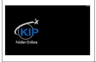
When Connected to the KIP Printer, if this image is displayed on the Folder Screen the KIP Printer is controlling the folder in an online condition. In order to put the folder into an Offline state, at the touch screen of the printer select the **Folder Offline** button.
